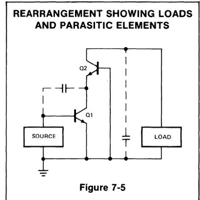
ground as in the circuit of Figure 7-3 and some feedback does occur. However, it is negligible because the collector of the first stage is heavily loaded by the emitter of the second stage. Therefore, very little feedback voltage may be developed across it. Figure 7-6 shows the circuit as it might be used. It has a gain capability greater than the circuit of Figure 7-3.
