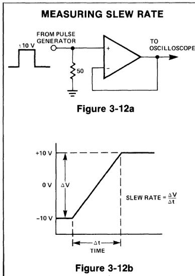
Figure 3-12 shows a typical bench set up for measuring the response of the output to a step input. The input step frequency should be of a frequency low enough for the output of the op amp to have sufficient time to slew from limit to limit. In addition,  $V_{in}$  must be less than absolute maximum input voltage and the wave form should have good rise and fall times. The slew rate is then calculated from the slope of the output voltage versus time or
