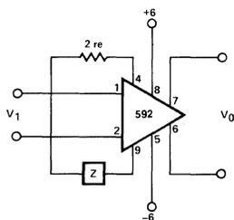
$$V_0(s) = \frac{1.4 \times 10^4}{Z(s) + 2re} V_1(s)$$
