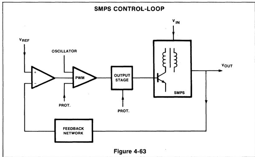
and load changes, the control module must give fast protection against overload, equipment malfunction, and the effects of switch-on immediately following switch-off. In addition the following features are desirable:
