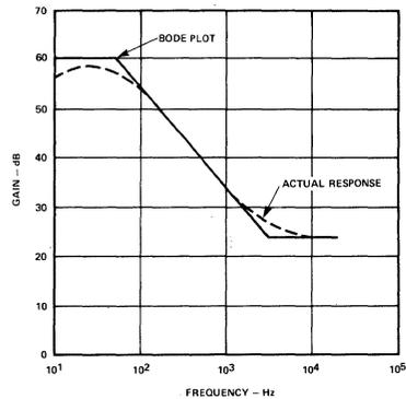
Bode Plot of NAB Equalization and the response realized in the actual circuit using the 531.
