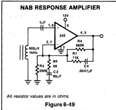
The lower corner frequency is determined next by the reactance of C4 and R4 such that:
