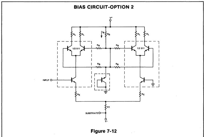
power supply required to bias the bases of the emitter-coupled transistors.
