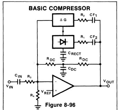
The same restrictions for the rectifier and ΔG cell maximum input current still hold, which place a limit on the maximum compressor output. As in the expander, the rectifier and ΔG cell inputs could be made common to save a capacitor, but low level tracking accuracy would suffer. Since there is no dc feedback path around the op amp through the ΔG cell, one must be provided
