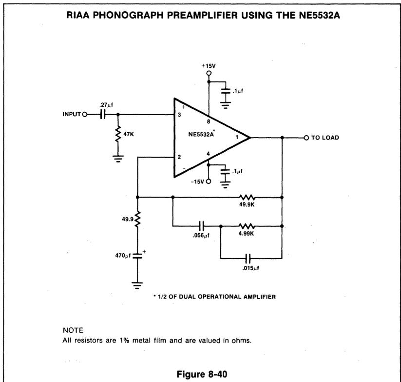
Signetics has recently introduced a new dual, low noise operational amplifier that is internally compensated to unity gain. It is called the NE5532. This dual operational amplifier comes in an 8-pin mini dual in-line package. It has the same characteristics as its single counterpart, NE5534.
