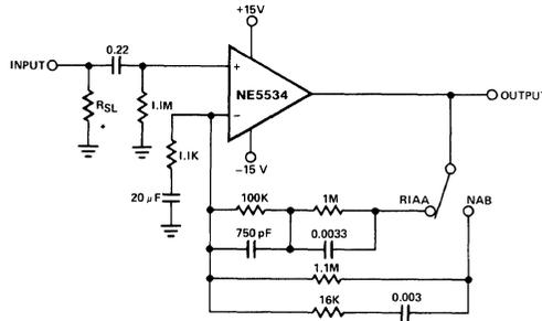
\*Select to provide specified transducer loading.
