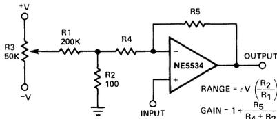
$$\text{RANGE} = +V \left( \frac{R_2}{R_1} \right)$$
