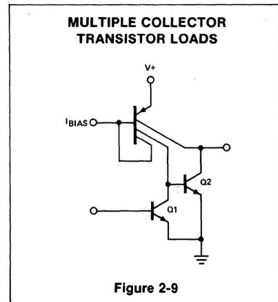
This circuit could give a voltage gain of many millions, which for linear amplification would be generally impractical due to clipping. A practical realization would incorporate feedback to define gain, as shown in Figure 2-10, where the voltage gain is given by the ratio:
