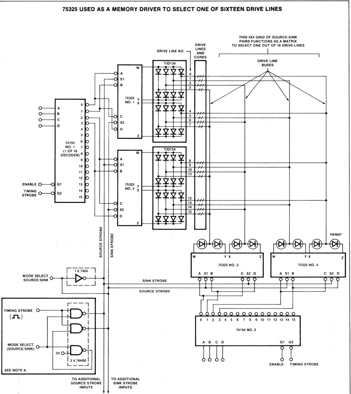
NOTE A This optional mode select and timing strobe technique can be used in place of the 7440 mode select and 74154 timing strobe when minimum time skew is desired.
