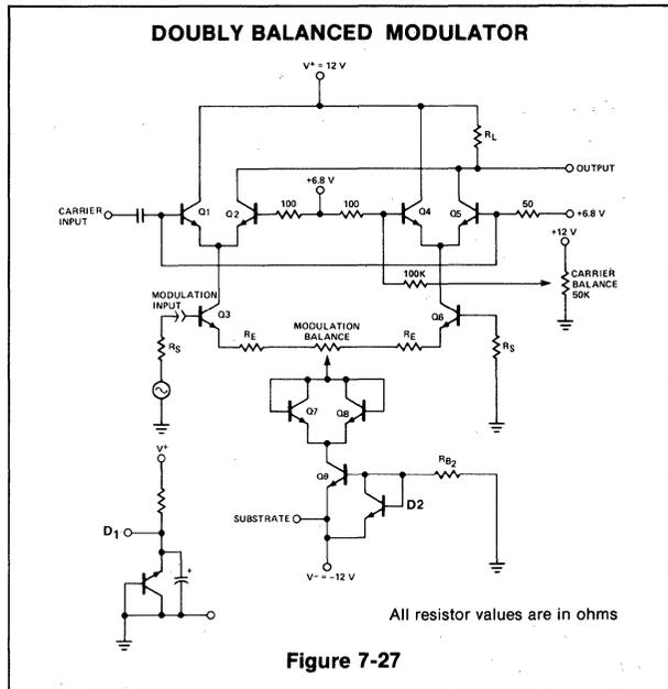
leaving the remainder of the circuit configuration unchanged. The lower half of a 511 is merely a current source. It may be replaced with a current source constructed from a discrete transistor or if differential modulation input is available, a resistor.
