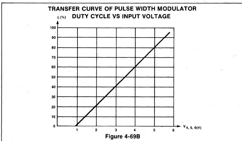
graph is given in Figure 4-69B. The output of the PWM causes the resetting of the output bistable.
