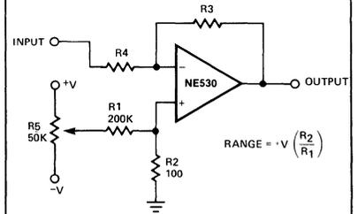
$$\text{RANGE} = -V \left( \frac{R_2}{R_1} \right)$$
