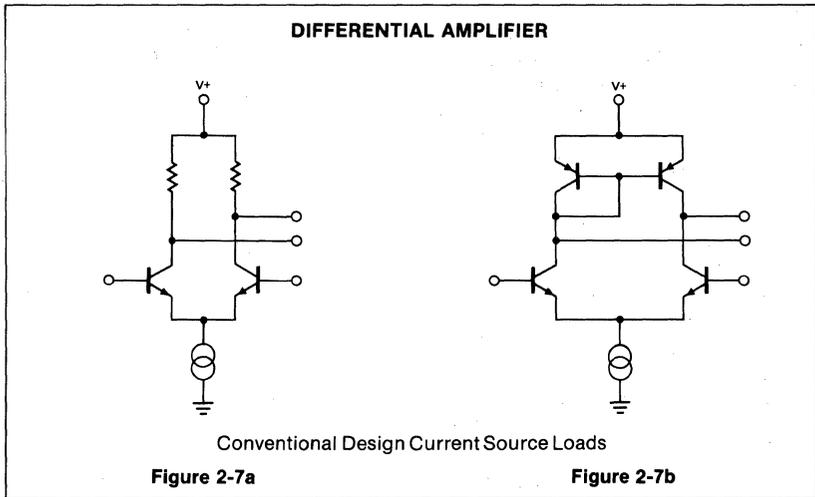
vantages of the circuit in Figure 2-7b are that the noise in the pnps is summed into the npn input noise, and the self-biasing scheme used in Figure 2-7b can introduce some added offset current if the pnp betas are low because pnps run at different current levels. A change in the circuit which avoids this problem is shown in Figure 2-8.
