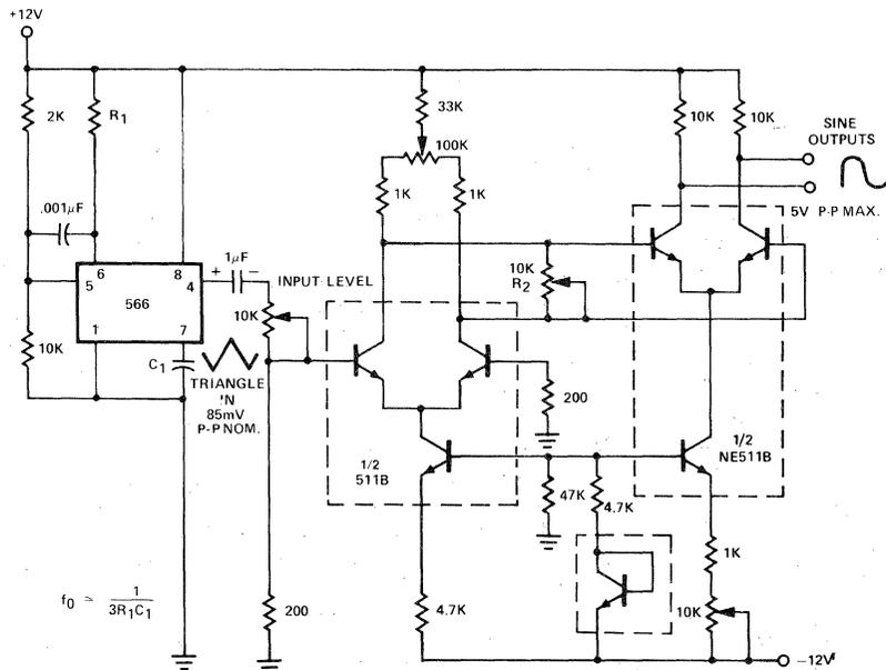
R<sub>1</sub>, R<sub>2</sub>, AND INPUT LEVEL MAY BE ADJUSTED TO GIVE LESS THAN 2% T.H.D. AT OUTPUT USING HEWLETT-PACKARD 333A DIST. ANALYZER.
