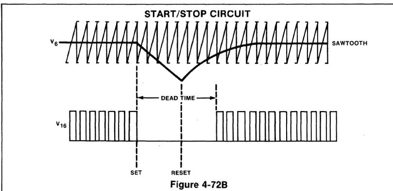
The operating frequency is not affected, because the upper trip level for sawtooth
