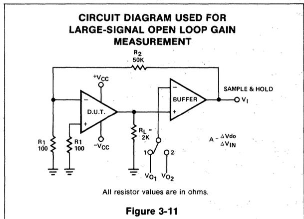
This operation is equivalent to swinging both inputs over the full common mode range, and holding the output voltage constant, but it makes the  $V_1$  measurement much simpler.
