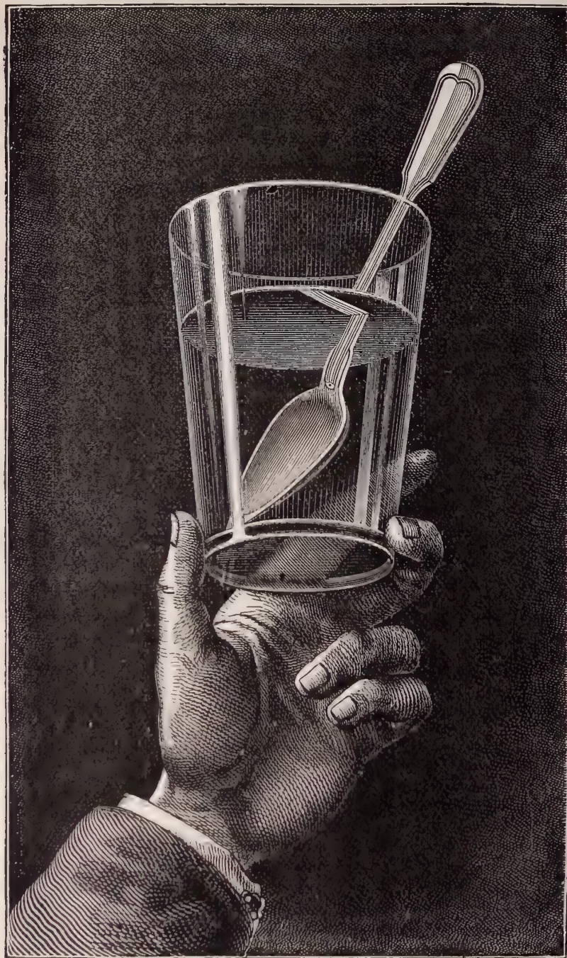
FIG. 3.—The phenomenon of total reflexion. (From the 'Forces of Nature,' published by Macmillan.)
