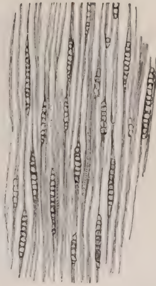
FIG. 490.—Portion of vertical section of the same wood, taken in a tangential direction, so as to cut across the medullary rays.
