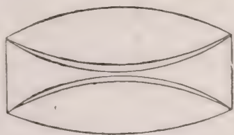
FIG. 267.—Tully's achromatic triples.
