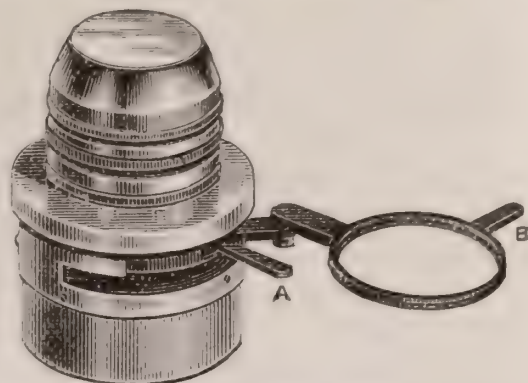
FIG. 200.—Powell and Lealand's new low-power condenser.
